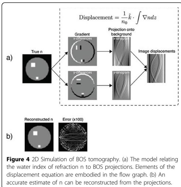
**Figure 4** 2D Simulation of BOS tomography. (a) The model relating the water index of refraction  $n$  to BOS projections. Elements of the displacement equation are embodied in the flow graph. (b) An accurate estimate of  $n$  can be reconstructed from the projections.
