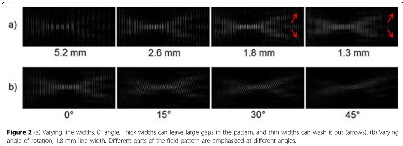
**Figure 2** (a) Varying line widths, 0° angle. Thick widths can leave large gaps in the pattern, and thin widths can wash it out (arrows). (b) Varying angle of rotation, 1.8 mm line width. Different parts of the field pattern are emphasized at different angles.
