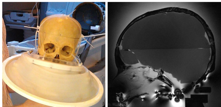
Figure 2 Bare skull strapped to holder (left) and as seen on MR T2w sagittal image (right).
