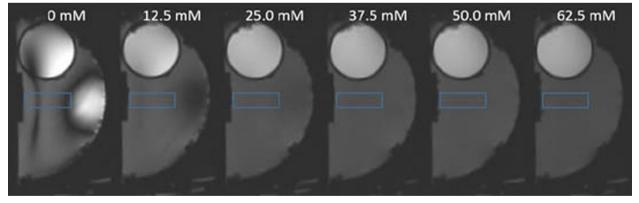
Figure 1 Side-by-side comparison of intensity images at different concentrations. Images show a sagittal view of an InSightec ExAblate 4000 head transducer with a water bath and head phantom.
