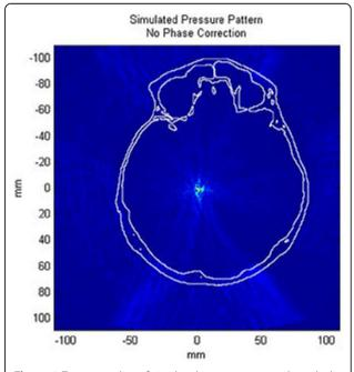
**Figure 1** Transverse slice of simulated pressure pattern through the skull with no phase correction employed. Skull is outlined in white
