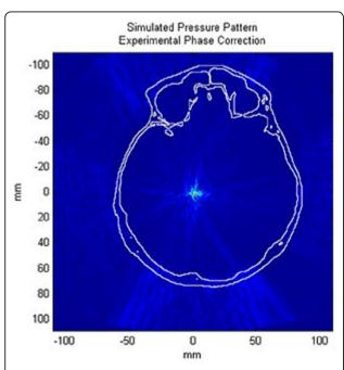
Figure 3 Transverse slice of simulated pressure pattern through the skull with experimentally employed phase correction. Skull is outlined in white
